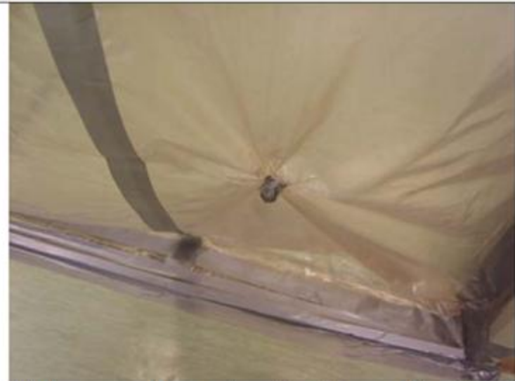
Make a small opening for air sampling by the H 2 O 2 detector, Portasens
