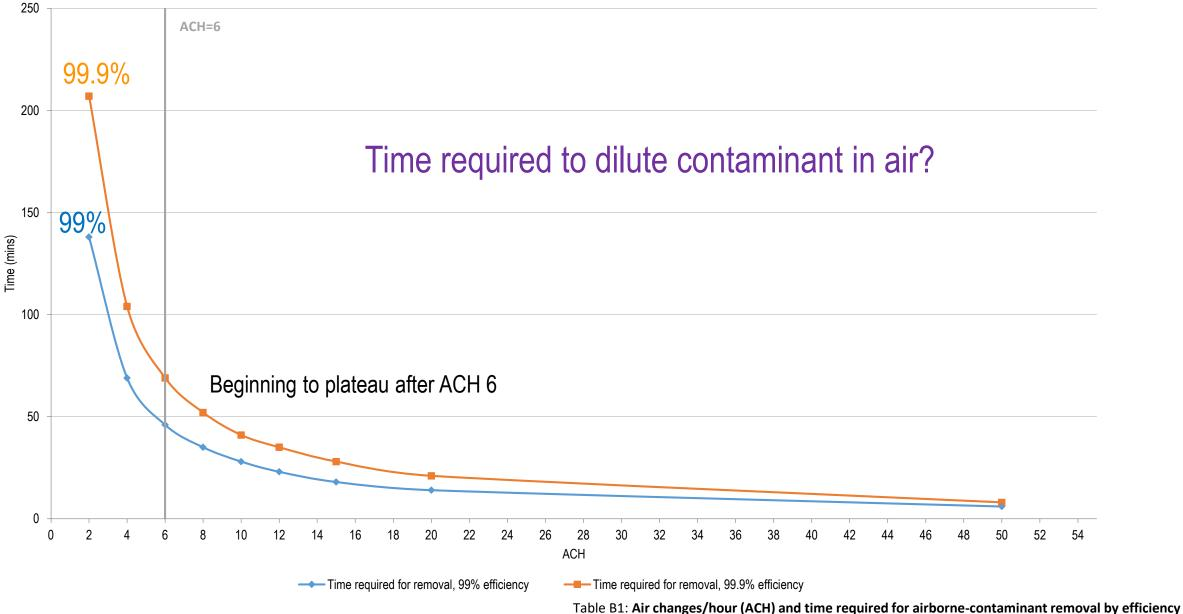
Air changes/hour (ACH) and time required for airborne-contaminant removal by efficiency
