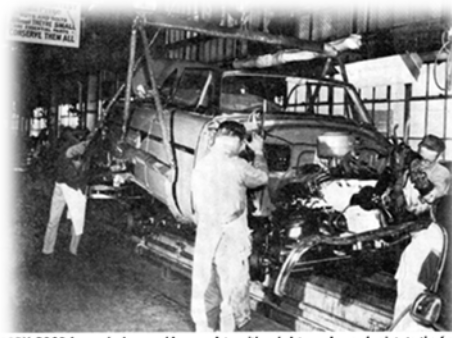
BODY DROP lowers body assembly, complete with upholstery, glass and paint, to the frame chassis employees (from left) Jim Young, Donald Hellmuth and James Graham take care to ensure the quality assembly for the addition of fenders and hood along the final line.
