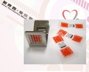
Load check indicator is an indicator printed with a pattern off test soil on both sides off a plastic see-through substrate.
