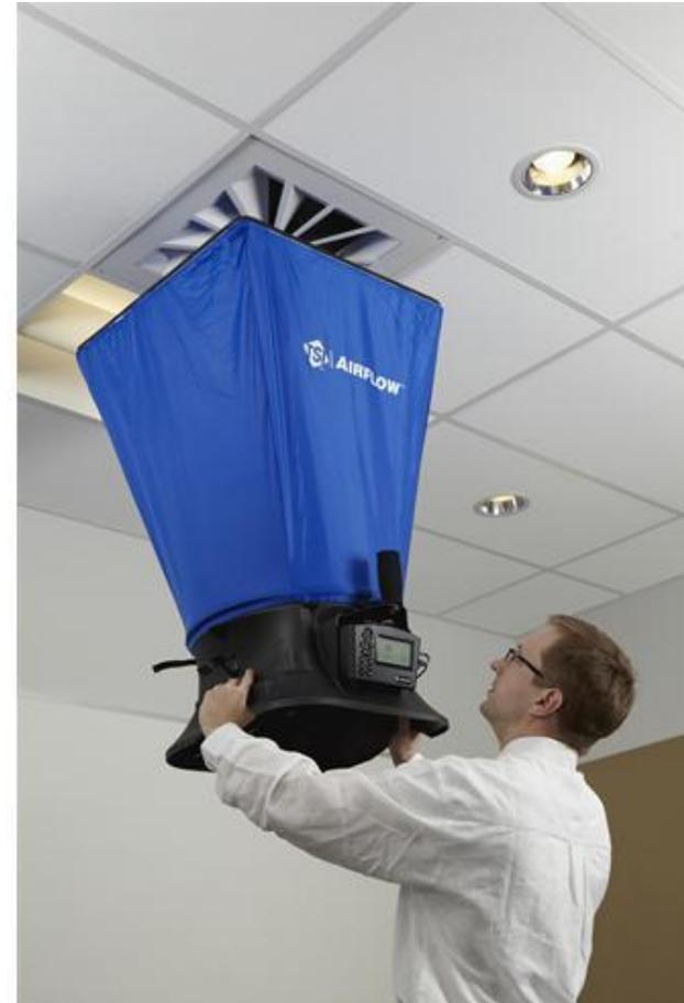
**TSI 8380 AccuBalance Air Capture Hood Balometer Manometer**
